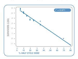
**TABLE 2.** MICROBIAL EFFICACY OF THE OZONE STERILIZER ON MICROORGANISMS EXPOSED TO THEIR KILLING DOSE (LESS THAN THE HALF CYCLE)
